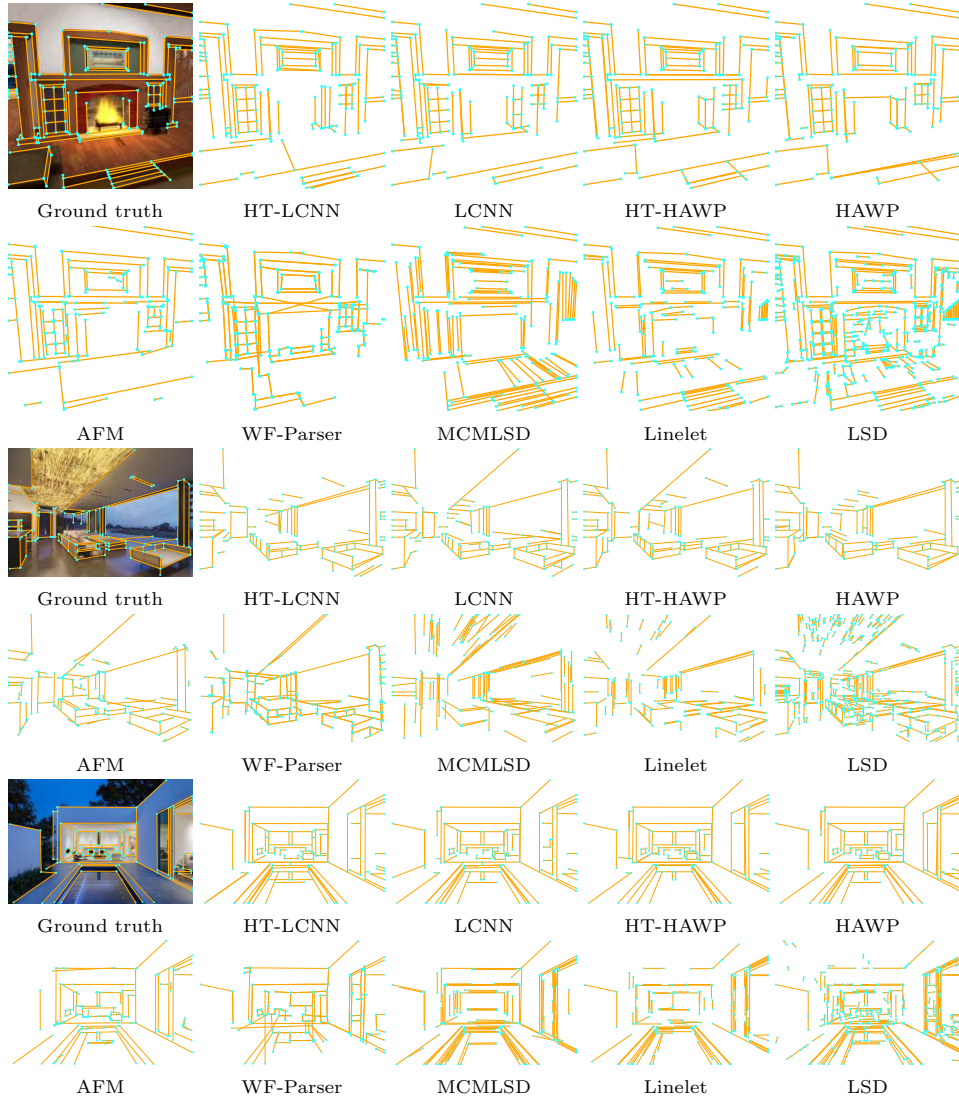
Fig. 13. Exp 3.(b): Visualization of detected line segments on the Wireframe dataset [18]. We show predictions from our HT-HAWP, HT-LCNN, and seven other leading methods: HAWP[52], LCNN [54], AFM [51], WF-Parser [18], MCMLSD [1], Linelet [7] and LSD [44]). (Continued on the next page.)
